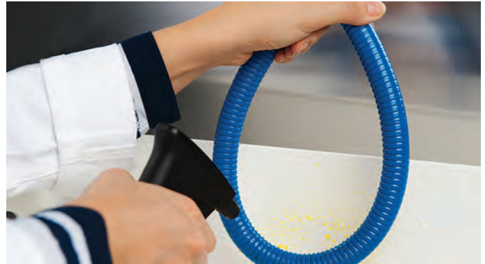
1. Spraying a solution of Riboflavin over a length of the conduit.
